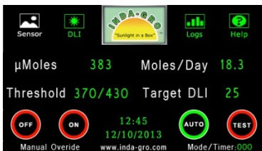
Main Sensor Screen – Manual & Test Override of programmed settings
